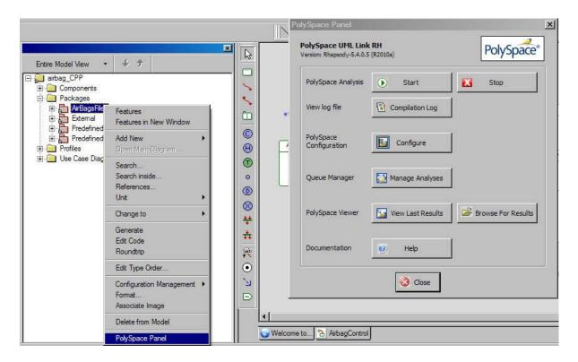
The PolySpace Panel has various button options that allow you to set up and perform PolySpace functions.
